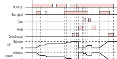
Start signal enables timing (timing is stopped when the start signal is OFF or when the power is OFF)
