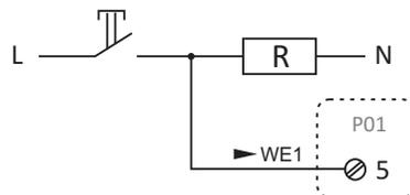
Example of connecting the receiver to the controlled output 1 for the remote control.
