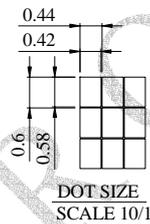
The non-specified tolerance of dimension is  $\pm 0.3$  mm.
