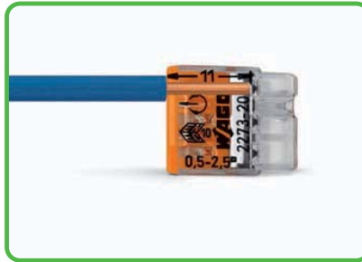
Strip solid conductor to 11 mm / 0.43 in (see marking).
